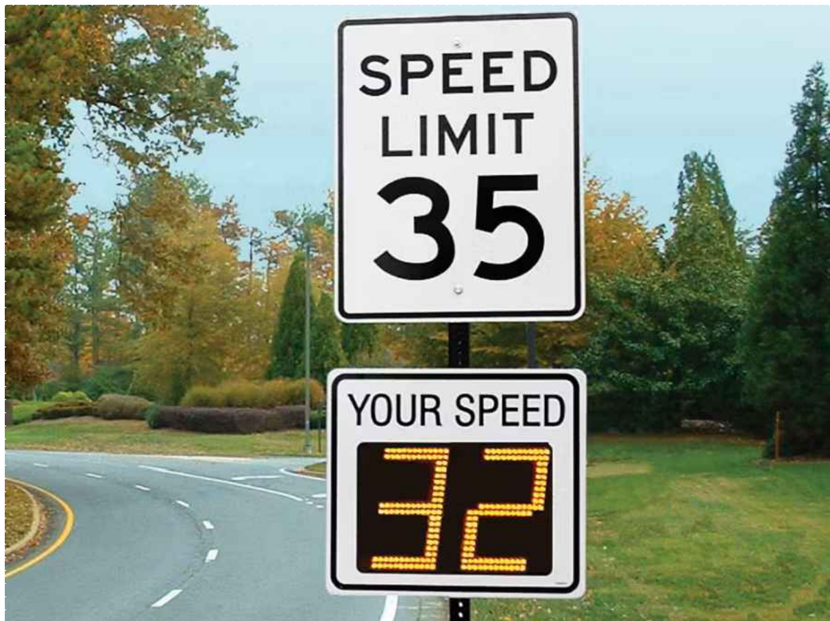
⑤ RADAR SPEED FEEDBACK ILLUMINATED SIGNS THAT USE RADAR TECHNOLOGY TO MEASURE THE SPEED OF APPROACHING VEHICLES AND PROVIDE THEIR ONCOMING SPEED. THE FEEDBACK SIGN IS PAIRED WITH A SPEED LIMIT SIGN, WHICH HELPS DRIVERS IDENTIFY IF THEY ARE TRAVELING ABOVE THE POSTED SPEED LIMIT.
