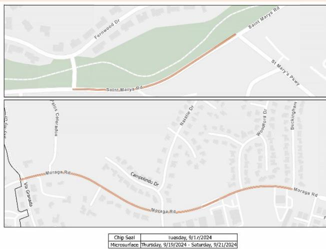
The Town's pavement project is now focusing on applying a rubberized cape seal Moraga Road and St Mary's Road. The rubberized cape seal consists of 2-part pavement preservation treatment: 1) microsurfacing seal; over 2) rubberized chip seal.
